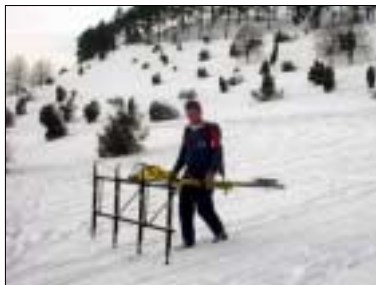
FEREX 4-probe gradiometer in the field
